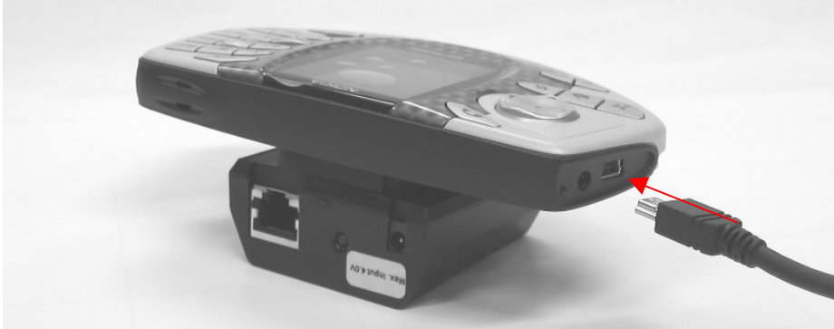
Figure 3: Mini-USB connector end of the cable is connected to Nokia N-Gage.
