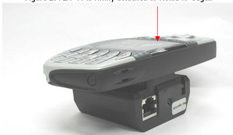
Figure 2: FLA-41 is firmly attached to Nokia N-Gage..
